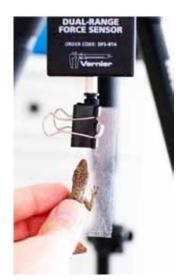
The gripping strength of a lizard is measured with this apparatus. Lizards with larger toepads were able to grip more strongly.
