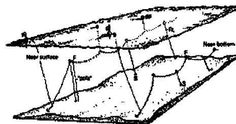
Fig 2: Semi-pelagic longlines with "near bottom" line on the right and "near top" on the left
