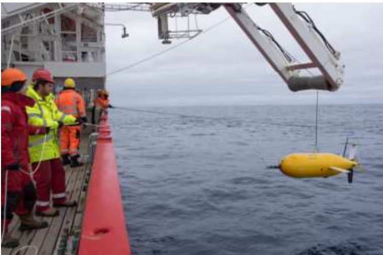
Boaty McBoatface (Autosub Long Range) during its first Antarctic deployment into the Weddell Sea off RRS James Clark Ross (Photo: British Antarctic Survey)
