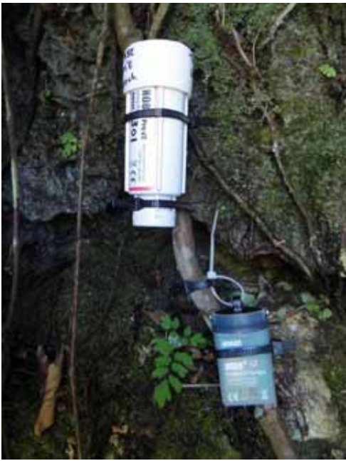
Figure 7. Environmental monitoring data-loggers at Church Cave. The HOBO U23-001 (top) records temperature and relative humidity, the HOBO UA002-64 (lower) records relative light intensity.
