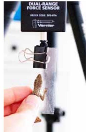
*The gripping strength of a lizard is measured with this apparatus. Lizards with larger toepads were able to grip more strongly.*
