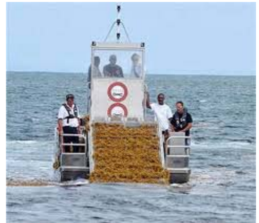
Specialised barge for removing sargassum from water Hinds et al 2016
