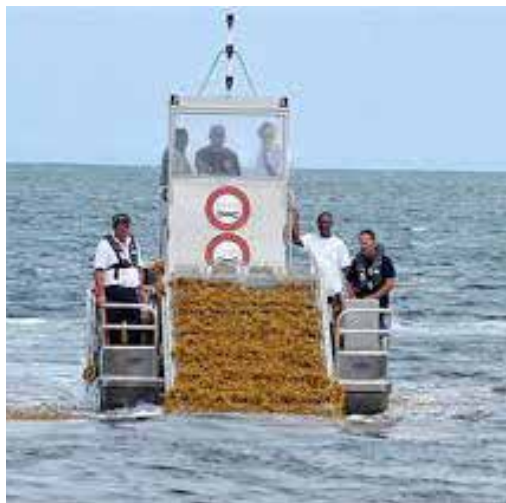
Specialised barge for removing Sargassum from water: Hinds et al 2016
