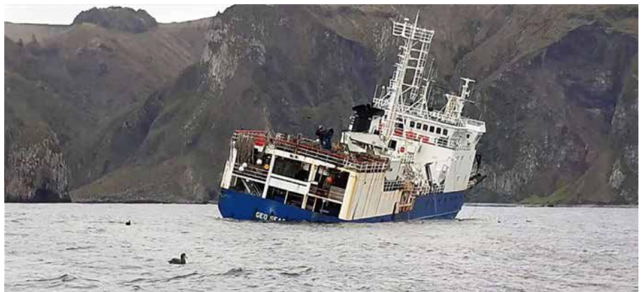
The MFV Geo Searcher down at the stern and listing severely as she sinks off Gough Island. Source: Tristan Government and Tristan Association website.
