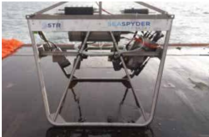
Deep water camera, able to function at a depth of 3000m
